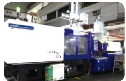
Injection moulding machine with hydraulic servo control
